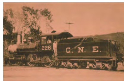
Above: C.N.E. #226 at Salisbury, Ct, headed toward Canaan. BLW#14276 1895 4-4-0 18"x24" 69". Old ND8C #8, later CNE #38, scrapped March, 1925.
