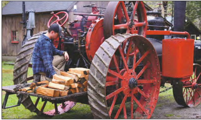
Left, wood fuel is loaded into an Eclipse steam engine as the machine fires up.
