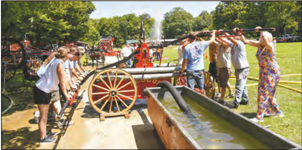
Handtubs involve hand pumping water from a tub to spray water out of a hose.
